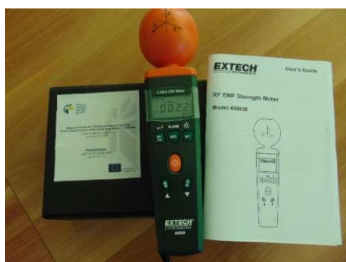
Fig. 5 – Measurements made with RF EMF Strength Meter - Model 480836
